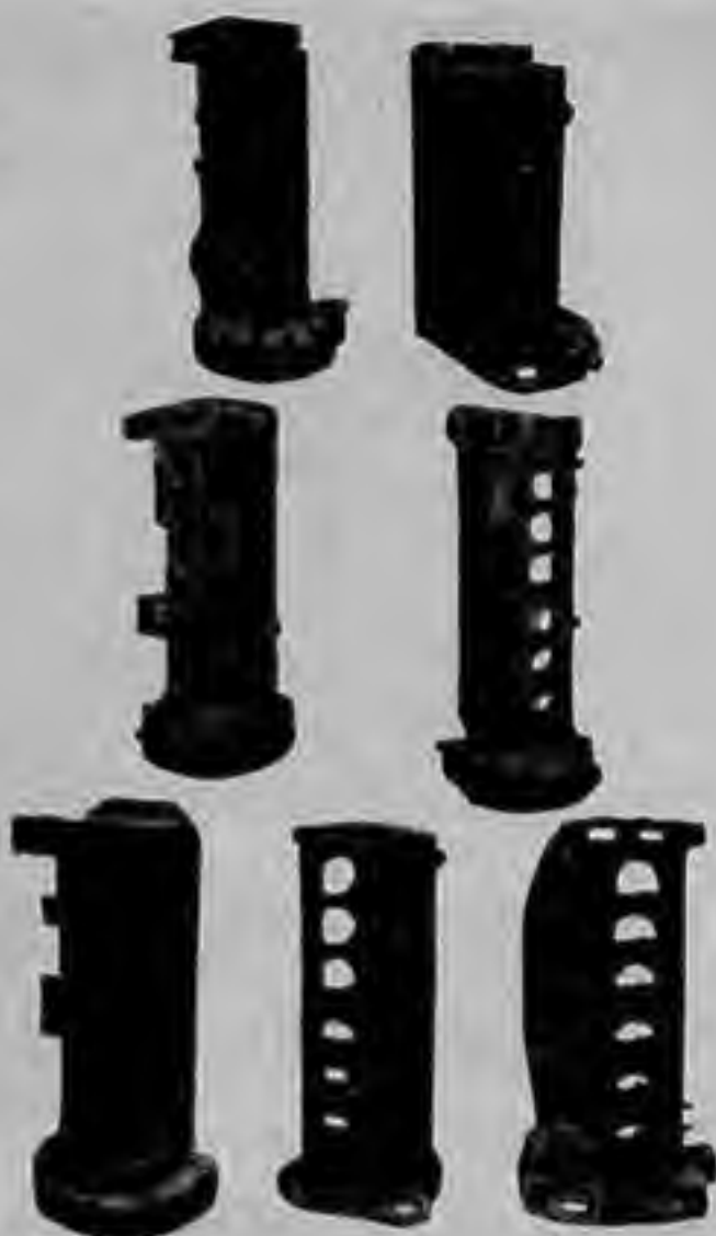
Fig. 1b.—Typical 6-cylinder commercial vehicle crankcases, for petrol and oil engines, cast in Elektron magnesium alloy. The weight of the largest casting is 168 lbs.; a similar casting in aluminium alloy would be 284 lbs.
